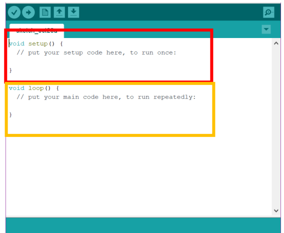
Figura 27: Void setup i Void loop
